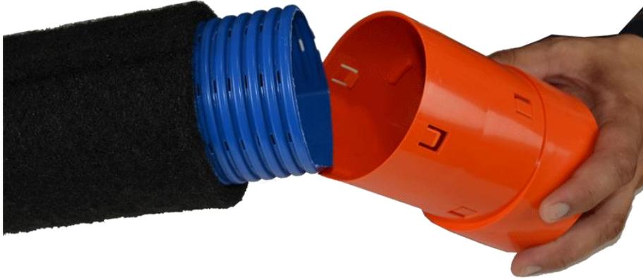
In order to install the **BATIFIBRE** sleeve on to the drain, position the flat part of the sleeve so that it is aligned with the drain channel, as shown in figure 17.
