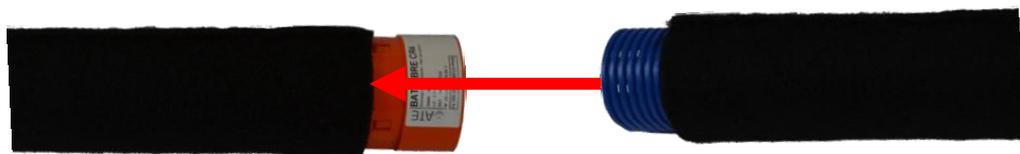
**FIGURE No. 16: COUPLING THE DRAINS BY INTERLOCKING**
