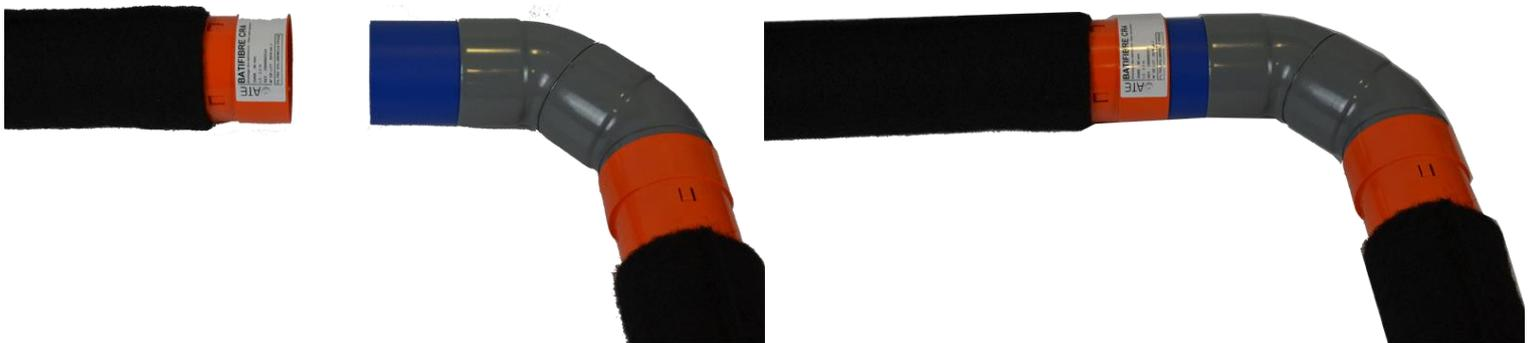
**FIGURE No. 23: CONNECTING THE **BATIFIBRE** DRAIN WHEN CHANGING DIRECTION BY 90° USING TWO MF PVC Ø100 45° ACCESSORIES**
