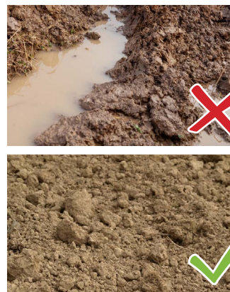
FIGURE 22: PRESENCE OR ABSENCE OF MUD IN THE BACKFILL
